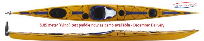
WIND 585 - Very fast, tonnes of storage, stable and given its length turns amazingly well. Ask someone who has paddled one. Length: 585 cm - Width: 54 cm - Carbon/aramide Weight: 24-26 kg - Retractable skeq+rudder
